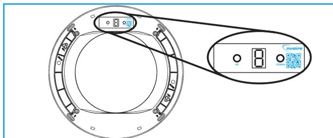
To use the remote monitoring device, the unique RFID code of each fan unit to be monitored must be known. Nuaire recommend that the RFID code is obtained at installation stage and recorded for use at a later date. The RFID code may be obtained by following the steps shown below.
