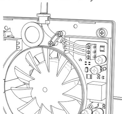
8 Cable Installation For Recessed Cable Entry
