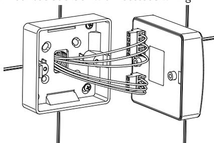
13 Recess mounted using metal backbox (not supplied)
