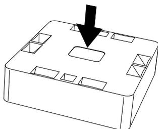
12 Surface mounted backbox with surface mounted wiring
