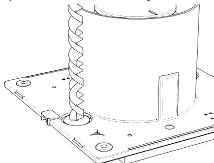
6 Remove Cable Gland For Surface Cable Entry
