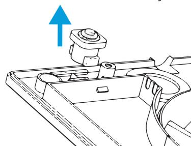
7 Cable Installation For Surface Cable Entry
