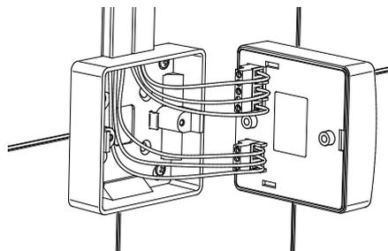
10 Surface mounted backbox with recessed wiring
