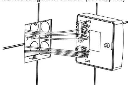
11 Select and breakout suitable apertures for surface wiring
