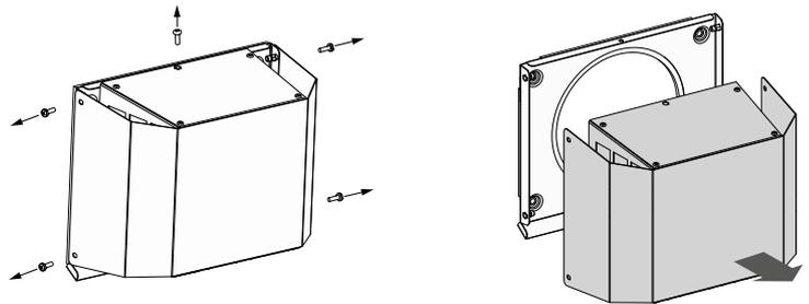
4. Fix the back part of the ventilation hood on the wall using the supplied screws 4x40.
