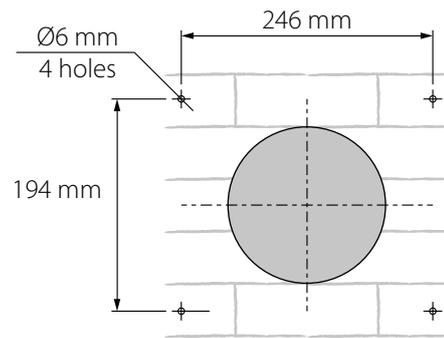
3. Insert the supplied expansion anchors 6x40 into the holes. Undo the 5 screws to remove the front part of the hood and to enable access to the fastening holes. For this undo the 5 screws and remove the ventilation hood front part.
